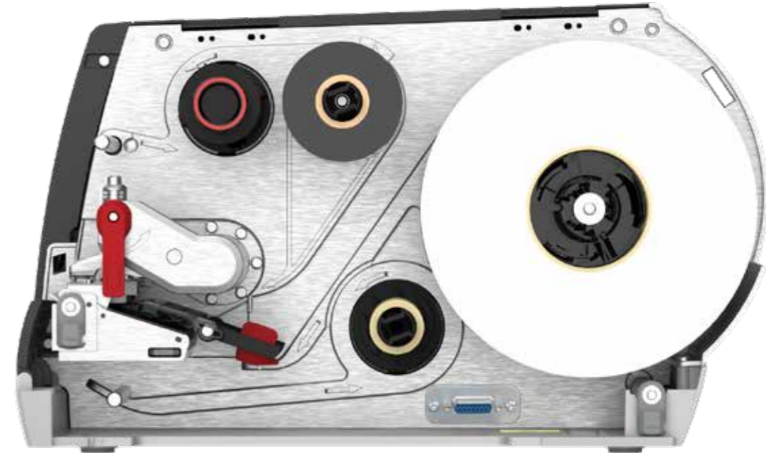
Rotating Media Hanger + Label Roll Core 76 mm (3.0 in) ID Shown with Label Roll 213 mm (8.38 in) OD Typical length of material with typical thickness of labels ~ 195 m
